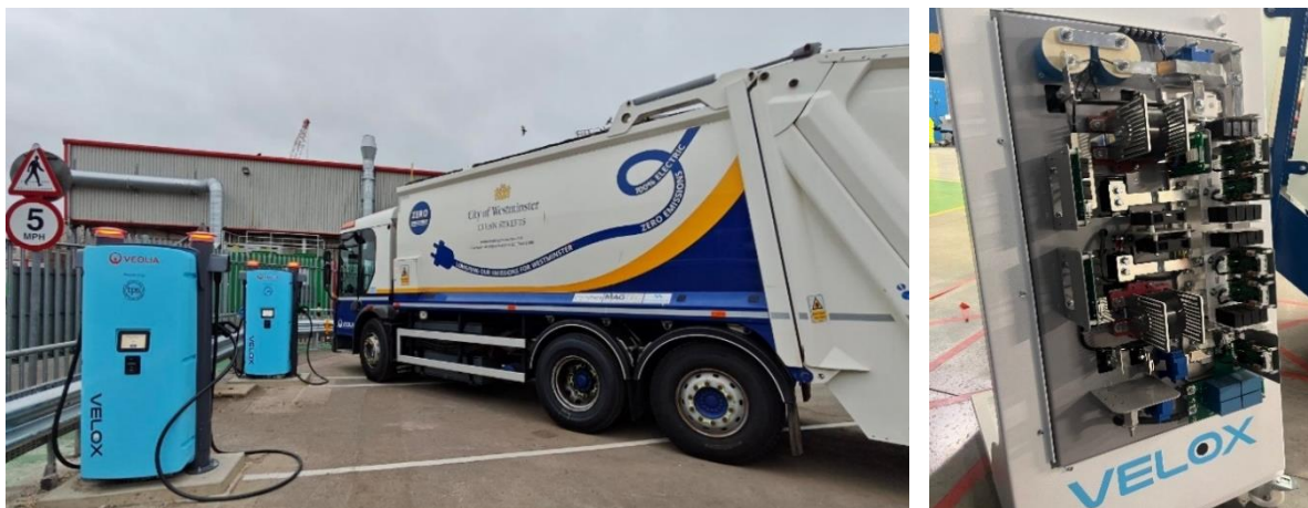
‘Velox’ V2X EV Chargers (Left) and their internal DC to DC power electronics with Silicon Carbide devices (Right)
